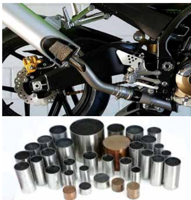
Figure 5. Catalytic converter installation and various product configurations.
