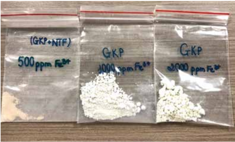
Figure 5. Images of the precipitates obtained from the mud acid mixture with different Fe contents.
