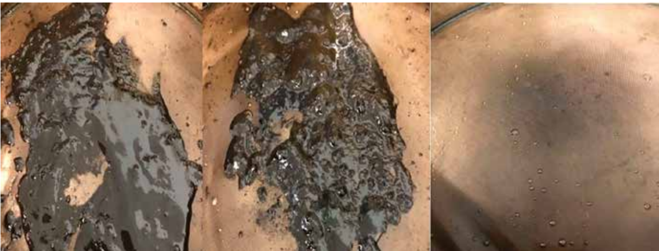
Figure 2. Images of samples (GKP acid and Well 1 crude oil mixture with different volume ratios) after passing through a 100-mesh screen.
