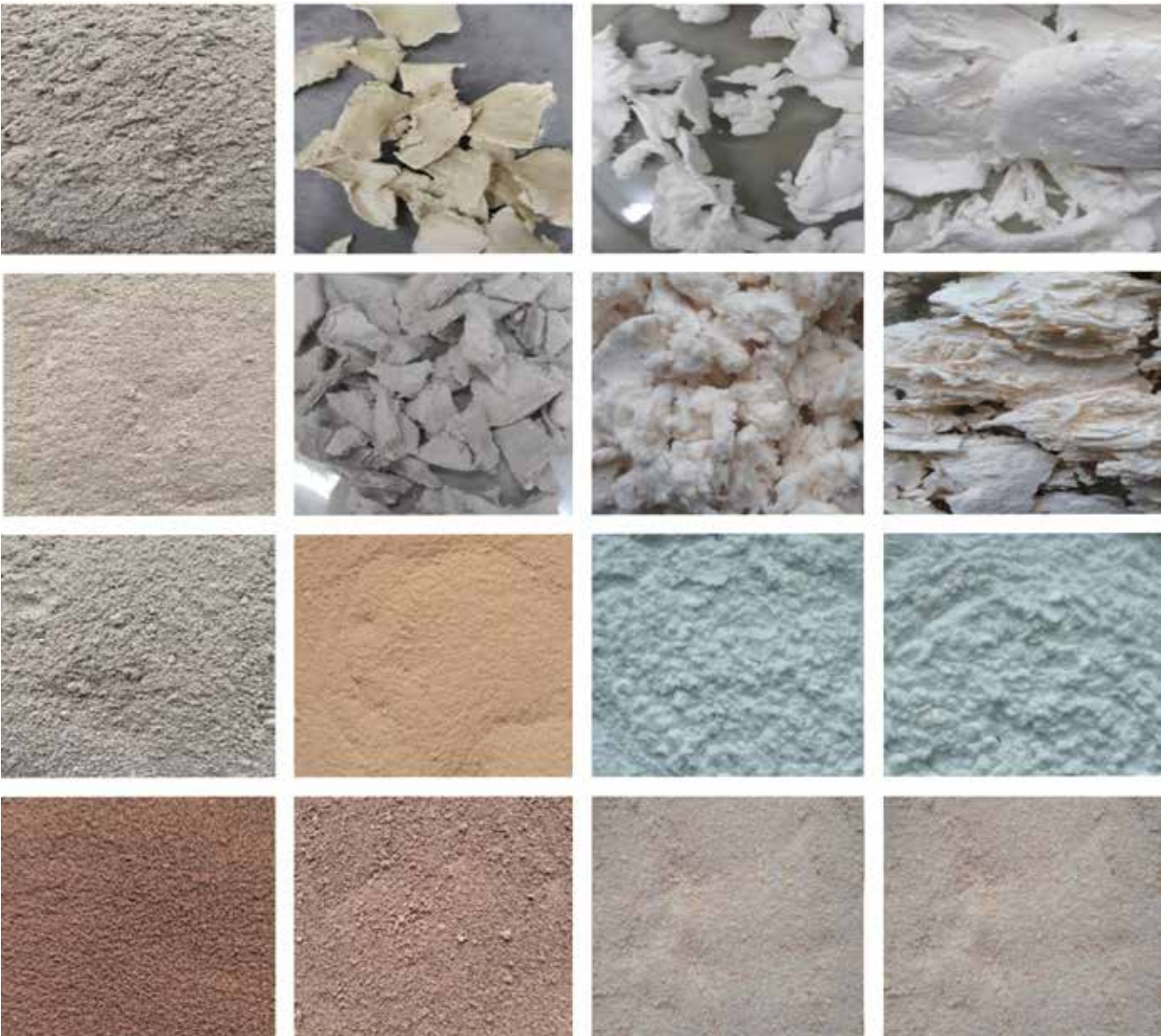
Figure 2. MCC extraction steps from various raw materials: from top to bottom - pineapple leaves, banana pseudostems, cassava stems, spent coffee grounds; from left to right - raw material powder, after lignin removal, after bleaching, and final MCC product.
