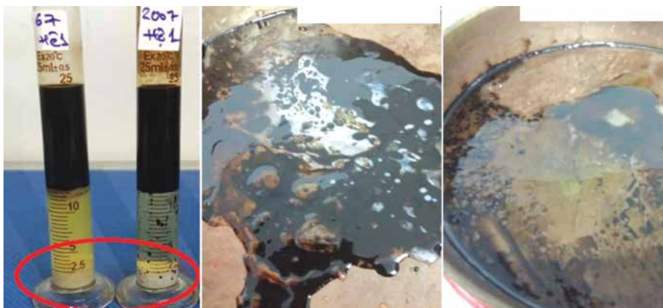
Figure 3. Images of precipitation and slug formation when CKP and GKP acid mixed with crude oil.
