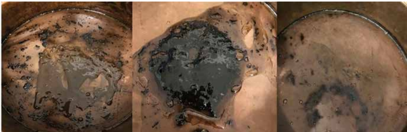
Figure 1. Images of samples (CKP acid and Well 1 crude oil mixture with different volume ratios) after passing through a 100-mesh screen.
